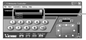
Select a camera for setting from the pulldown menu for the camera.
